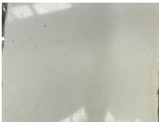
Figure 4.3 Example of aluminium painted surface exposed to a disinfectant repeatedly to disinfectant.
