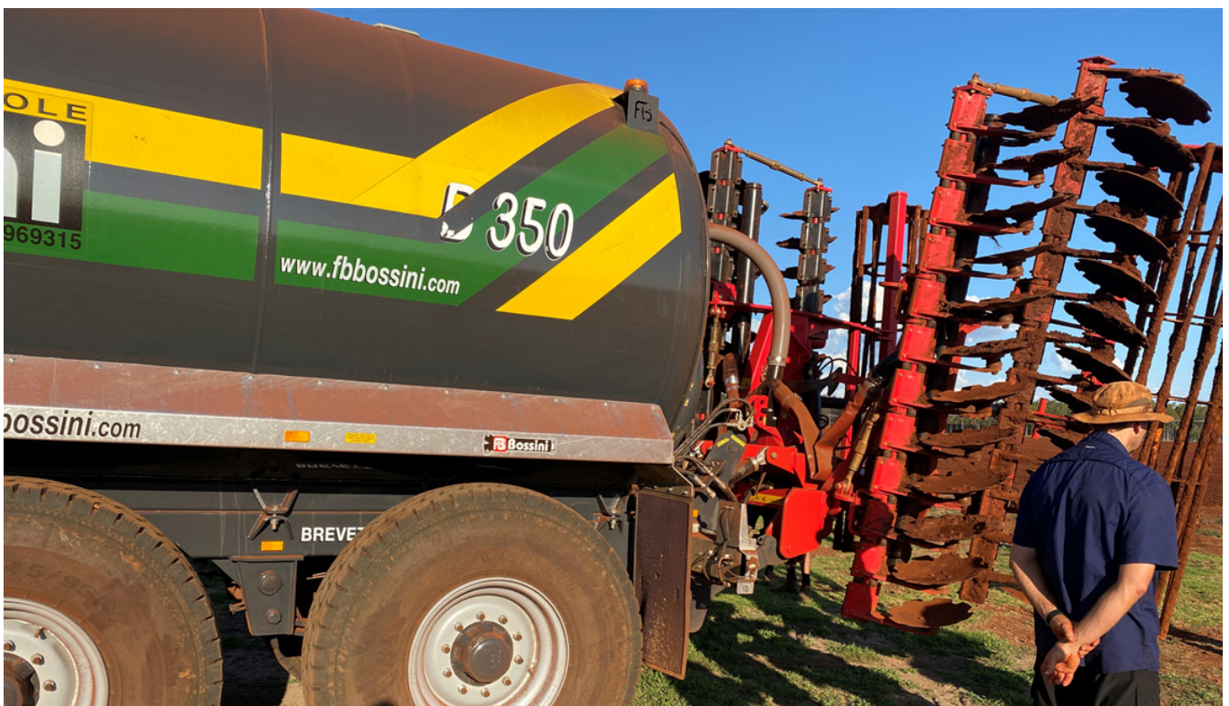
Figure 2. Direct injection slurry tanker with disc openers
