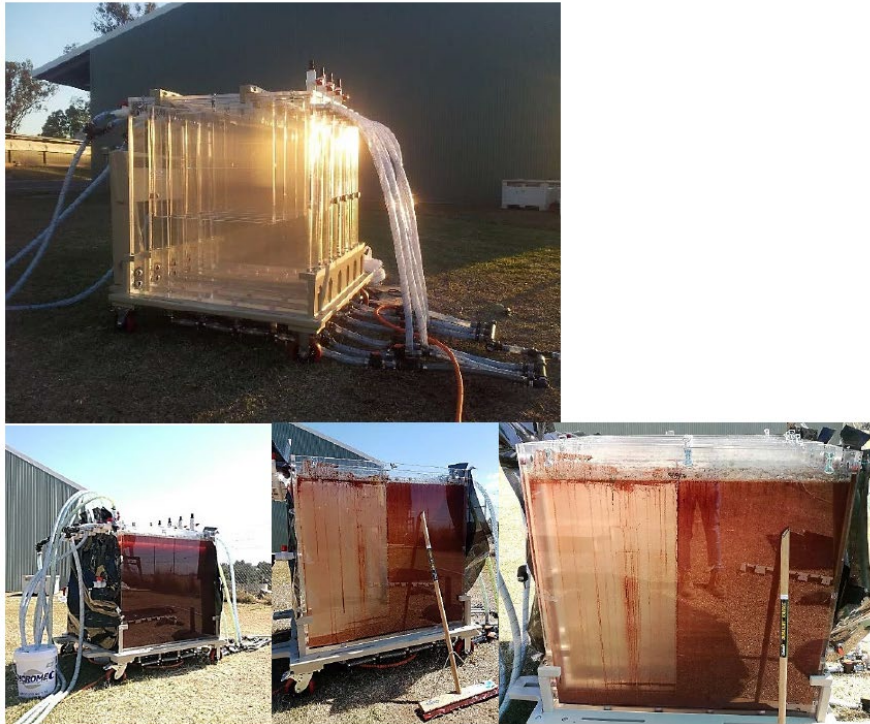
Figure 4. Schematic of flat-plate flow-through PPB reactor tank, (middle) a photo of the set-up prior to commissioning at the UQ Gatton piggery, and (bottom) a photo of the PPB biomass grown and harvested.
