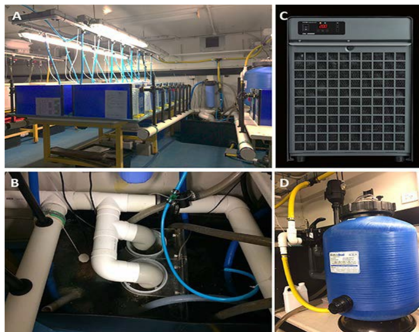
Figure 6. Fish tank infrastructure used in the testing of purple phototrophic bacteria (PPB) as a replacement aquaculture feed.
