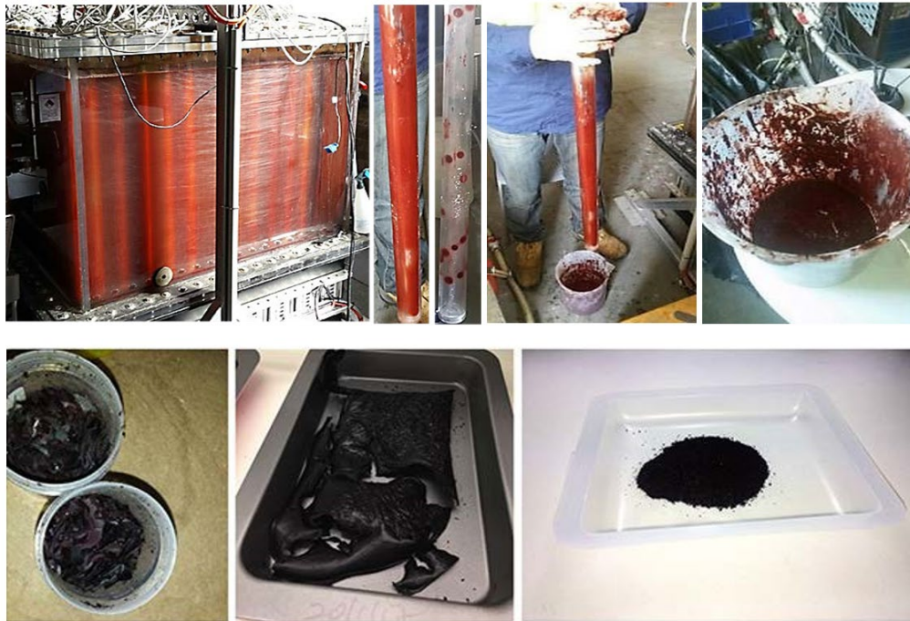
Figure 5. Manual harvesting and processing of purple phototrophic bacteria (PPB) from illumination tubes, and the resulting biomass at different stages of processing, in preparation for the fish feeding trial.
