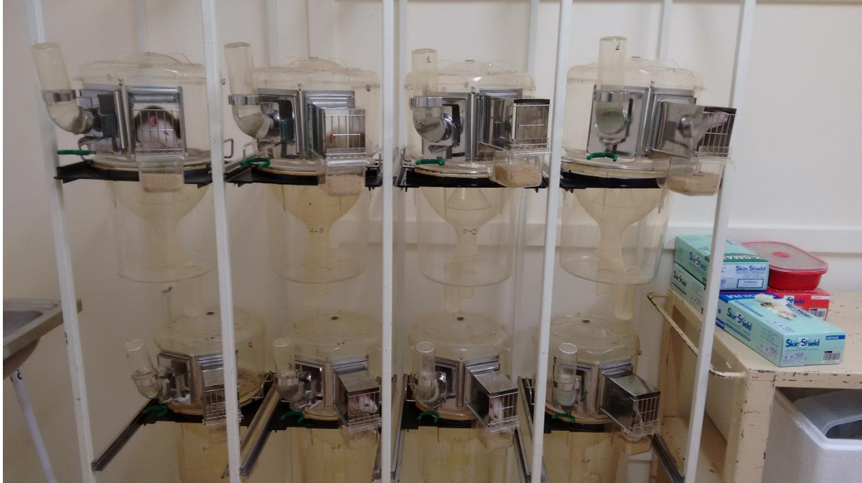
Image 1: Rat metabolic cages housed within a rack, rats within the cage have access to water and feed, two sample collection tubes are inserted from beneath the cage and the funnel cage design allows for the separation of faeces and urine.
