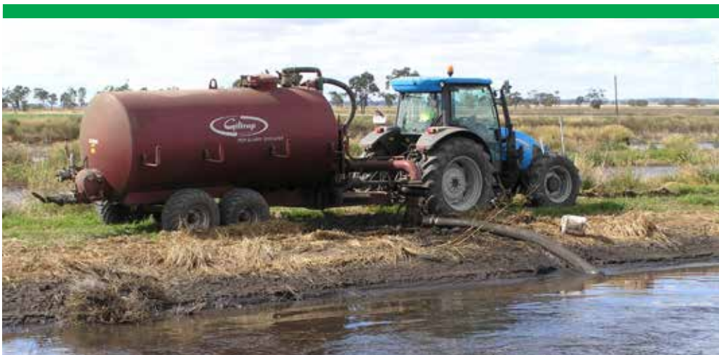
Photograph 22 Sludge removal using a vacuum tanker and agitation (Source: Alan Skerman, DAFF)
