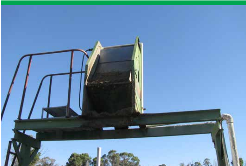
Photograph 7 Stationery rundown screen at piggery
