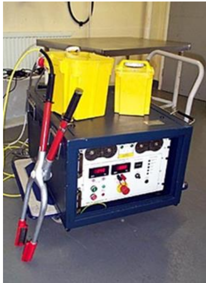
Figure 13. Electrocution equipment for pigs – 400-volt stunner
