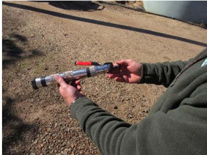
Figure 11. Medium size captive bolt gun – in-line, penetrating, cartridge ammunition
