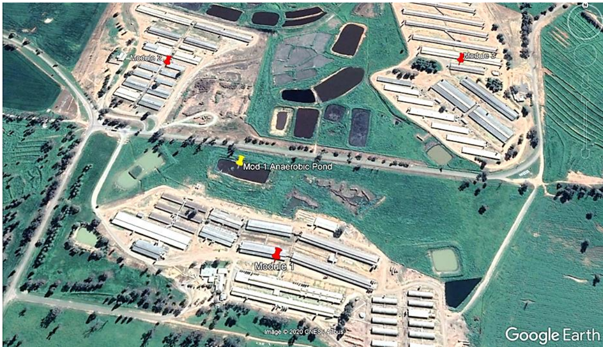
Figure 12 Aerial photograph showing existing uncovered “Mod 1 Anaerobic Pond”, which is proposed to be extended to form a new covered anaerobic pond that captures biogas from Module 1 and Module 2 onsite at the large piggery.
