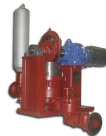
Figure 7: Komline-Sanderson plunger pump
