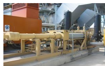
Figure 8: GEHO DHC valve operated hydraulic piston pump
