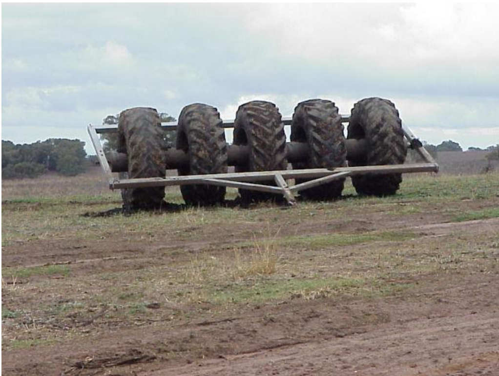
Photograph 25: Tyres used to break the surface crust to enhance solids drying in a SEPS
