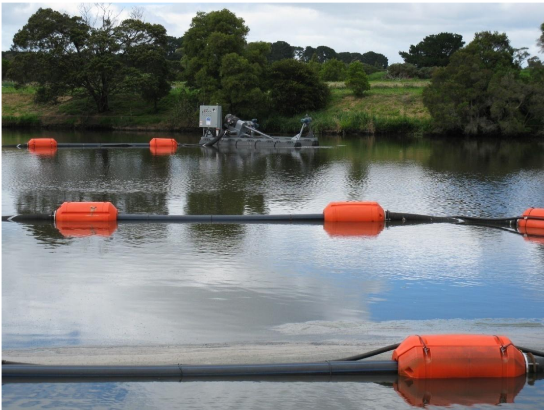
Photograph 12: Pond dredge in operation (Dredging Solutions)
