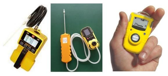
Figure 3.2 Typical portable biogas/hydrogen sulphide safety detectors (Google images)
