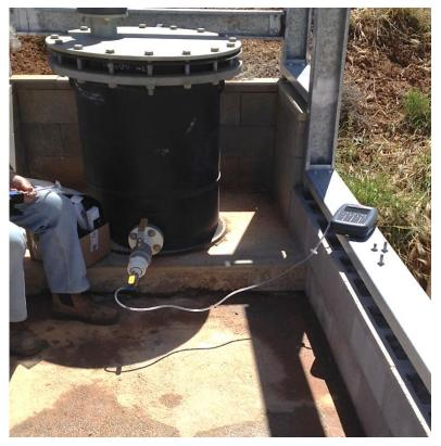
Figure 3.1 Measurement of biogas composition on-farm
