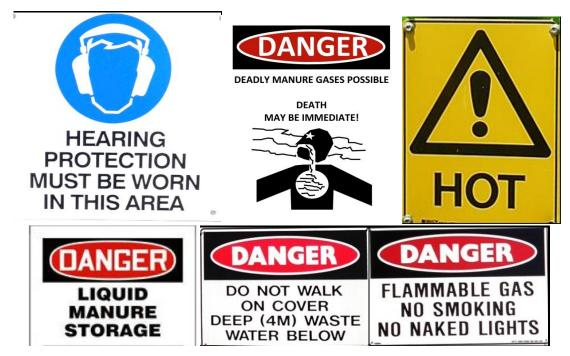
Figure 2.5 Typical safety signage around an on-farm biogas plant (Photos courtesy of the Pork CRC)
