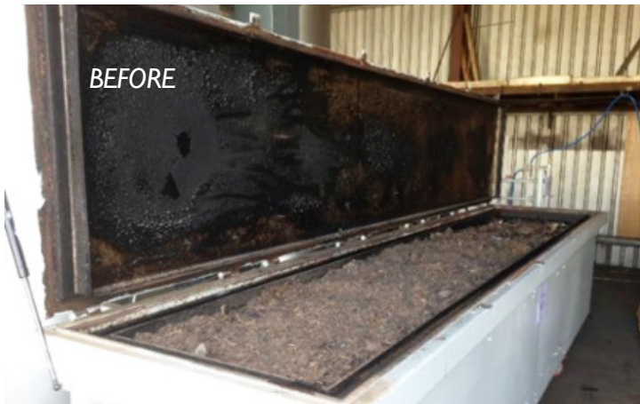
MIHG reactor before biomass is ignited
