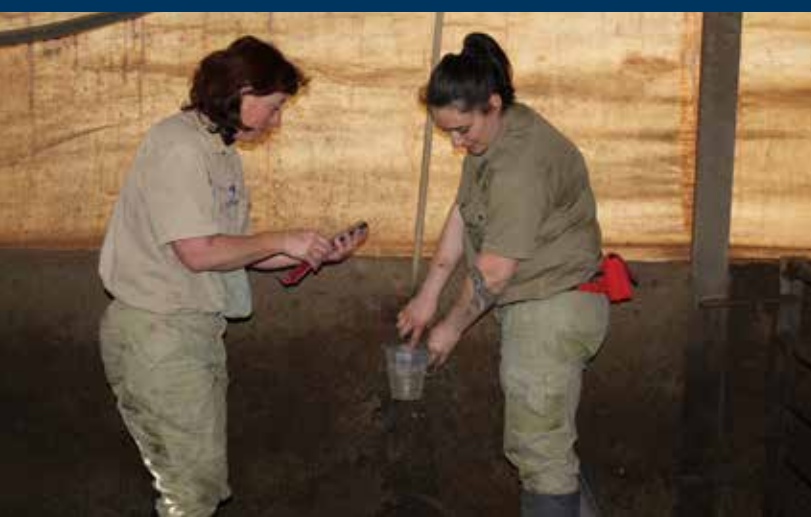
FIGURE 2: Measuring water flow rate in dry sow pen
