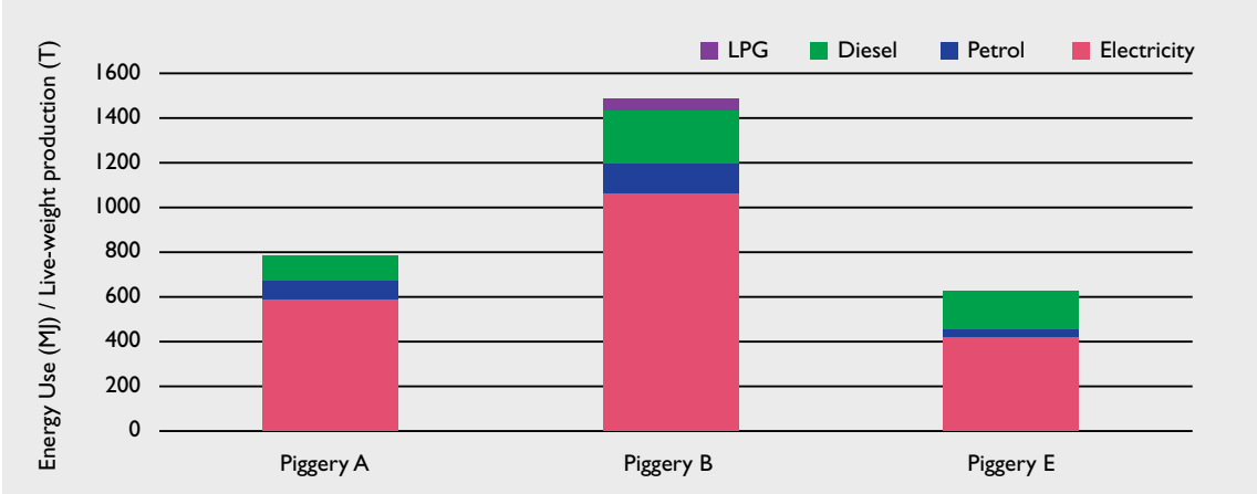
FIGURE 1 Energy Use (MJ) per Unit Liveweight Production (T) for Farrow to Finish Piggeries
