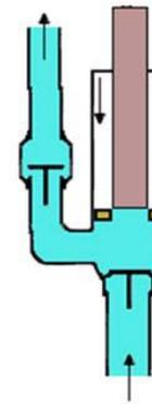
Double-acting, differential closed plunger pump
