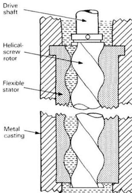
Figure 7 – Schematic of screw pump
