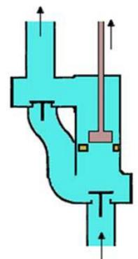
Figure 6 – Schematic of plunger pumps
