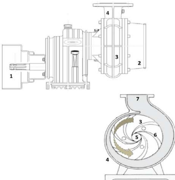
**Figure 1 – Centrifugal pump: 1 = power take-off, 2 = inlet with suction nozzle, 3 = impeller, 4 = volute case, 5 = suction nozzle, 6 = vane, and 7 = volute discharge (Brambilla et al. 2013)**
