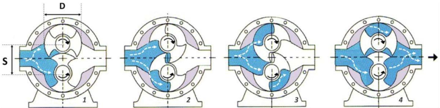
**Figure 9 – Example of rotary lobe pump and its operation ( $S$  = shaft diameter and  $D$  = tip diameter). Scimitar-shaped lobes are able to reduce build-up of particles between the rotors and the case**
