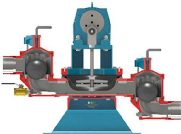
**Figure 3 – Schematic of GEHO-ZPM diaphragm pump**
