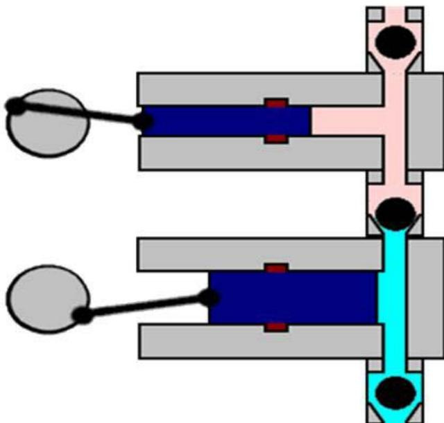
Figure 5 – Schematic of piston pump
