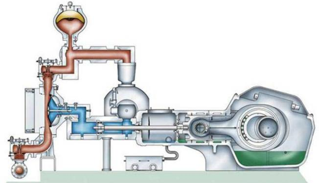
**Figure 4 – Schematic of Mud Sucker diaphragm pump**
