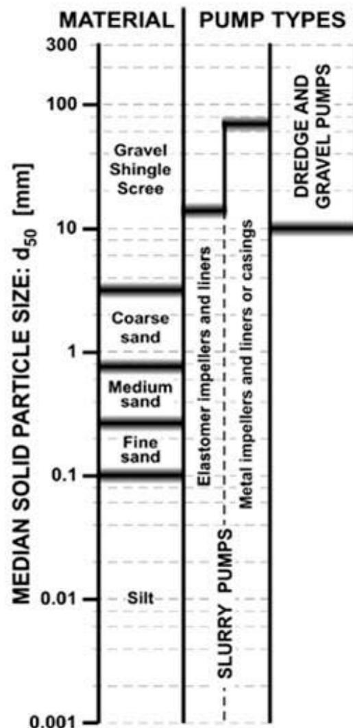
Figure 2 – Particle Size Pump Selection Guide
