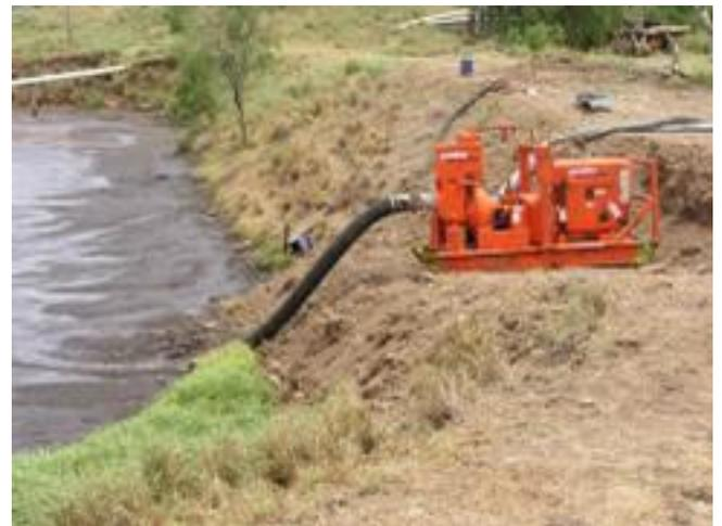
Figure 1 – Dewatering an anaerobic piggery pond
