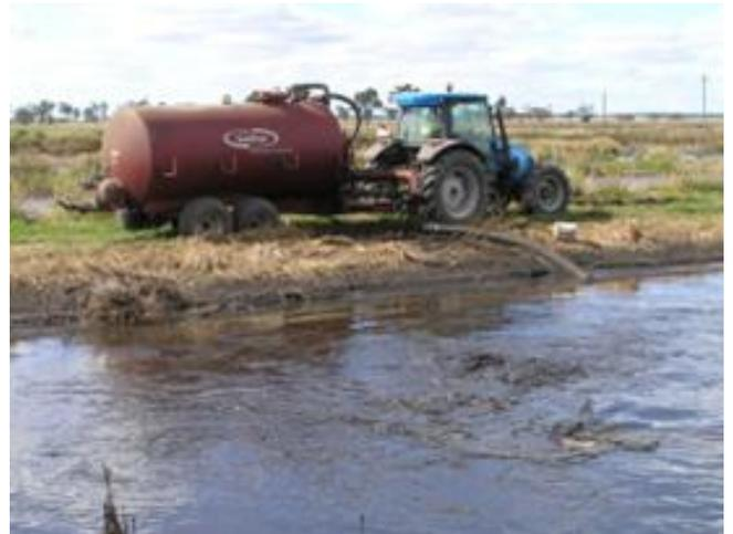
**Figure 3 – Sludge removal using a suction tanker with recirculating pump for agitation**
