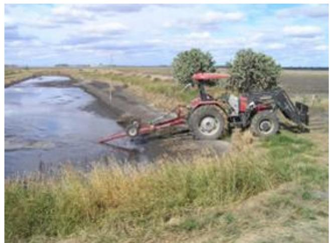
**Figure 4 – Tractor PTO driven pond agitator**
