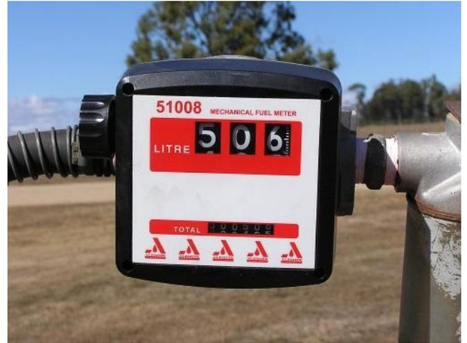
**Figure 7: Alemite Mechanical Flow Meter**
